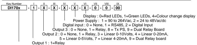
Input type: 1 = RTD or linear mV, 2 = T/C, 3 = Linear mA, 4 = Linear Volts
