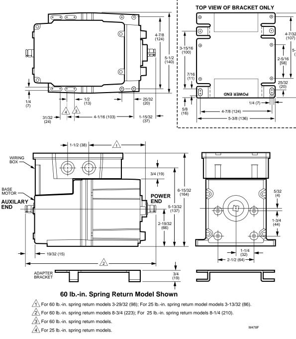
Fig. 1. M4185/M4186/M8175/M8185 mounting dimensions in in. (mm). NOTE: M4182/M8182 motors do not have auxiliary shaft, but all other dimensions are the same.
