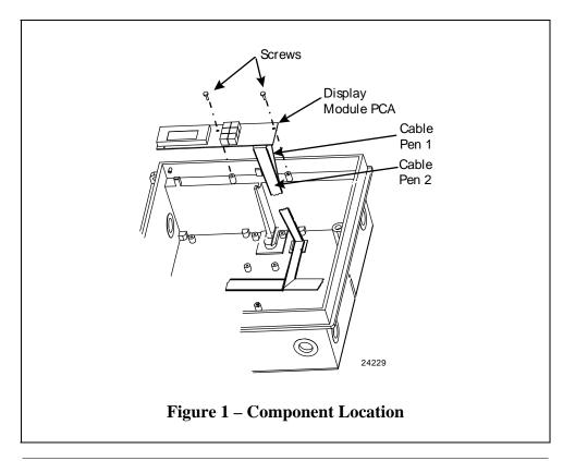
Installation Procedure Follow the procedure in Table 1 to install the new display module PCA in your recorder.
