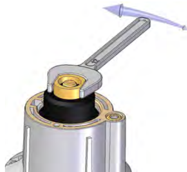
Figure 11 Adjusting flow rate.
