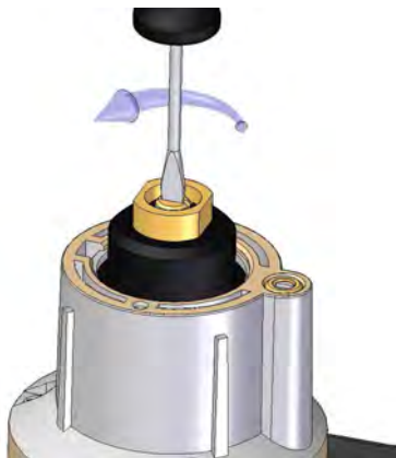
Figure 12 Adjusting step pressure.
