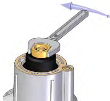
Figure 11 Adjusting flow rate.
