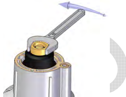
Figure 24: Adjusting flow rate.
