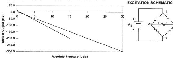
**TERMINATION** STYLE Style 6 - 1 x 4 Pin 1 = Vs (+)Pin 2 = Output (+)Pin 3 = Ground (-)Pin 4 = Output (-)Pin 1 is notched
