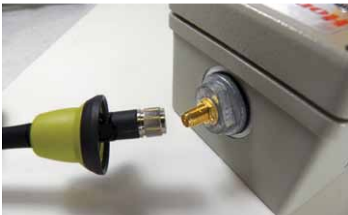
Figure 14. Limitless™ WOI RP-SMA Connection, Integral
