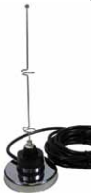
WAN10RSP straight mobile antenna, magnetic mount
