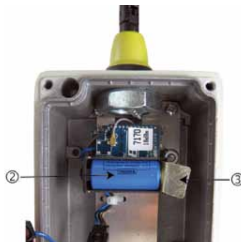
Figure 5. Limitless™ WOI Battery and Insulator
