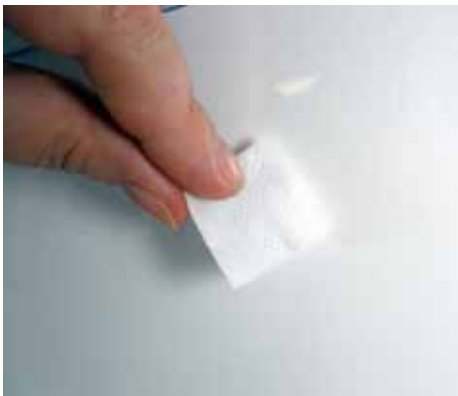
Figure 17. Adhesive Mount Antenna – Step 1. Pre-clean the surface
