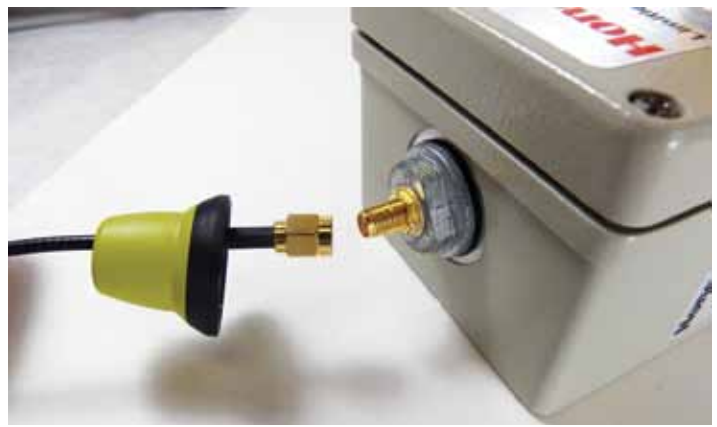
Figure 15. Limitless™ WOI RP-SMA Connection, Remote
