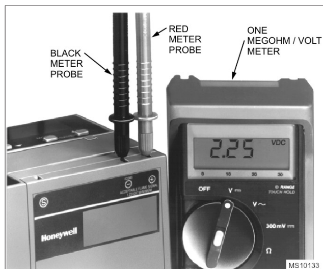
Fig. 11. Measuring voltage flame Signal with 7800 SERIES controls
