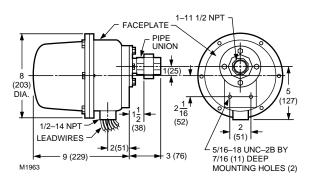
Fig. 2. Dimensions of C7012C and F in in. (mm).
