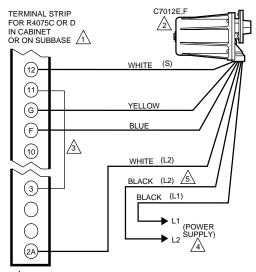
AN R7247C DYNAMIC SELE-CHECK AMPLIFIER MUST BE USED WITH AN R4075C OR D.
