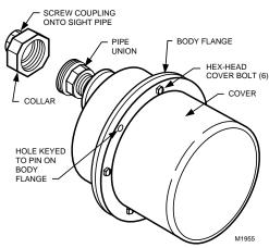
Fig. 8. Mounting C7012C or F Detector.
