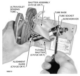
Fig. 20. Replacing ultraviolet radiation sensing tube.
