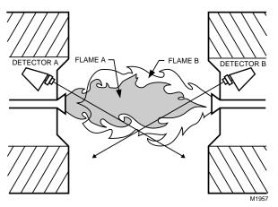
Fig. 4. Example of flame discrimination problem (opposed burners).
