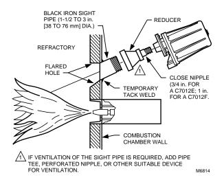
Fig. 5. Typical mounting of C7012.
