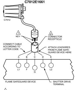
BOTH CONNECTORS ARE KEYED TO ALLOW CONNECTION IN ONLY ONE POSITION.
