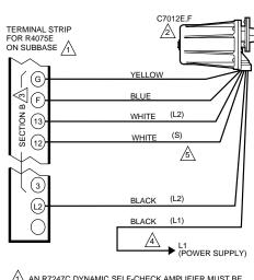
AN R7247C DYNAMIC SELF-CHECK AMPLIFIER MUST BE USED WITH AN R4075E.
