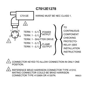
Fig. 16. Wiring connection for C7012E1161 or C7012E1278.
