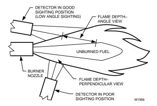
Fig. 3. Detector sighting angle.
