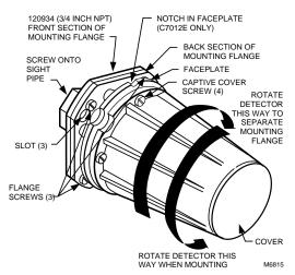
Fig. 7. Mounting C7012A, E, or G Detector.
