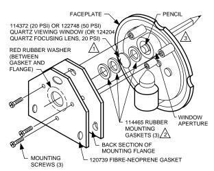
\(\frac{1}{\text{Liewing window can be replaced with either side toward the flame.}\)
