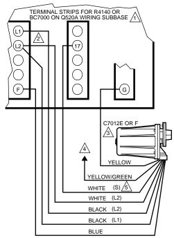
AN R7247C DYNAMIC SELF-CHECK AMPLIFIER MUST BE USED WITH AN R4140, BC7000.
