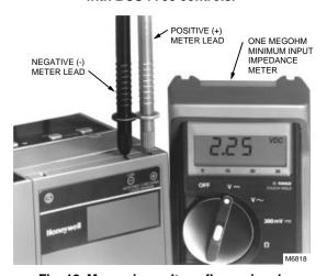
Fig. 19. Measuring voltage flame signal with 7800 SERIES controls.
