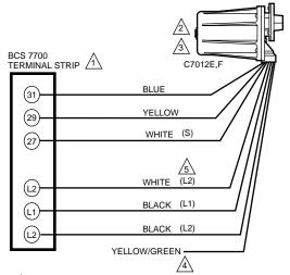
A R7747C DYNAMIC SELF-CHECK AMPLIFIER MUST BE USED WITH THE C7012E,F/BCS 7700 COMBINATION. SHUTTER CYCLE RATE IS 12 TIMES PER MINUTE. SUGGEST USING SERIES 7 OR GREATER FOR THESE APPLICATIONS.
