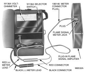
Fig. 17. Measuring microamp flame signal.
