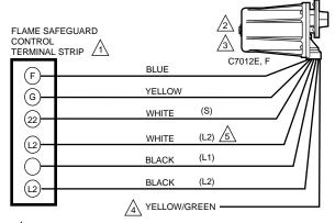
A R7847C DYNAMIC SELF-CHECK AMPLIFIER MUST BE USED WITH A 7800 SERIES FLAME SAFEGUARD CONTROL INCORPORATING THE SHUTTER DRIVE CIRCUIT. SHUTTER CYCLE RATE IS 12 PER MINUTE. SUGGEST USING SERIES 7 OR GREATER FOR THESE APPLICATIONS.
