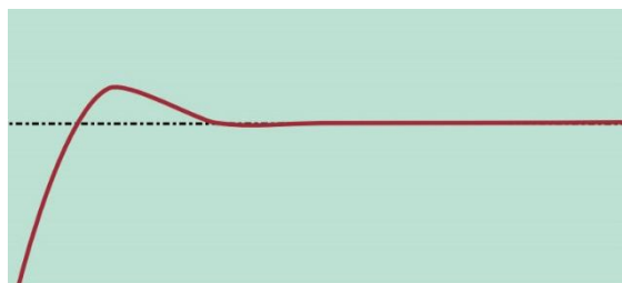
Too Small: Overshoots setpoint before settling
