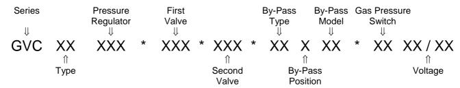
**Series**: GVC = combined valve unit <u>with</u> connection
