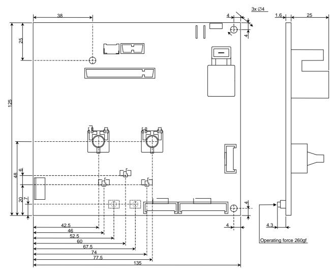
Measurement unit: mm – Tolerance:  $\pm$  0.2mm
