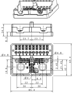
Socket NE Fig.3 Regarding the connection of the control units, provisions such as strain reliefs, sufficient earth terminals and neutral terminals should be present in the appliance or in external connection boxes.
