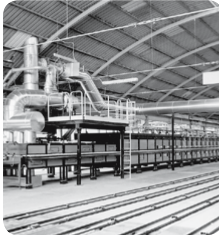
Roller hearth kiln in the ceramics industry
