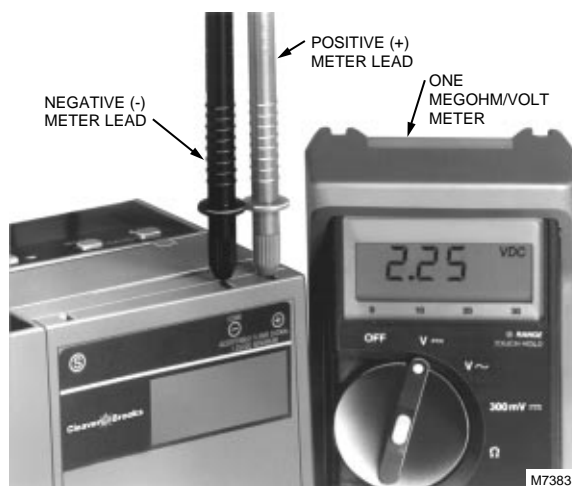
Fig. 22. Flame signal measurement.
