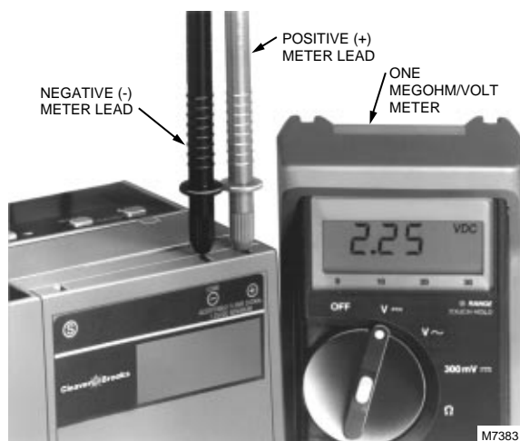
Fig. 22. Flame signal measurement.
