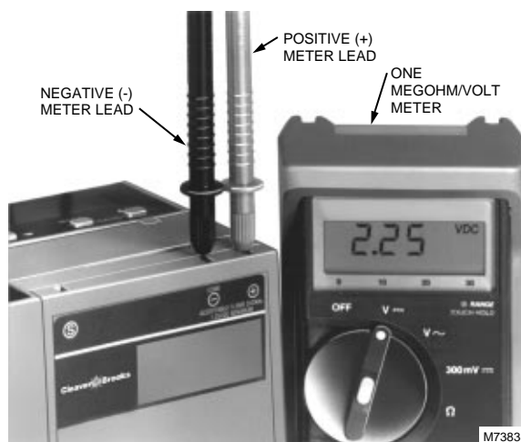
Fig. 22. Flame signal measurement.
