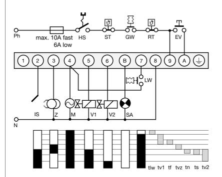
HS Mains switch GW Gas proving switch ST Limit thermostat RT Control thermostat
