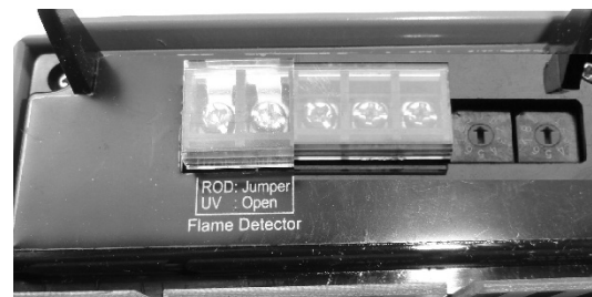
ULT Model (bus connector and address switches)
