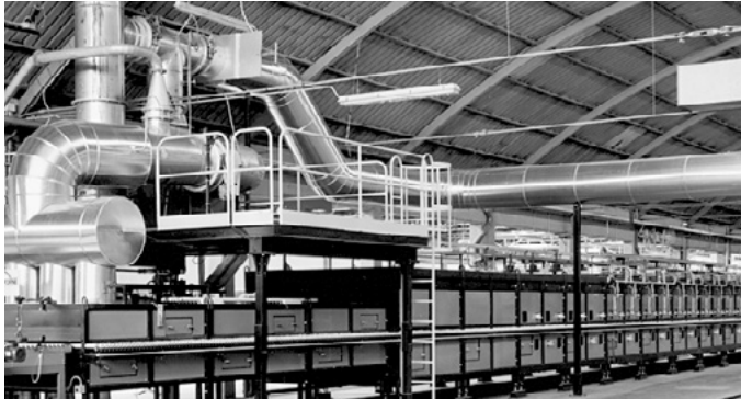
Roller hearth kiln in the ceramics industry
