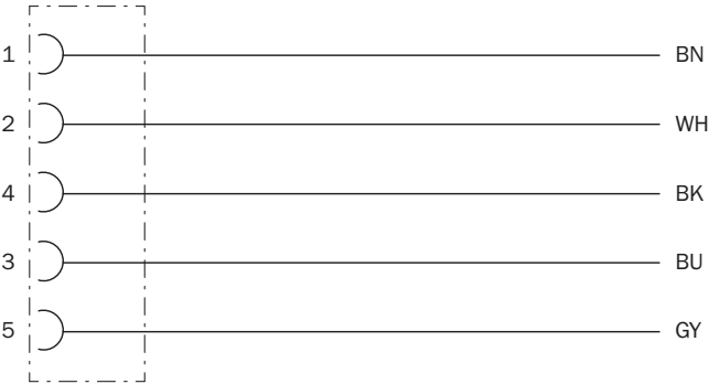
Contact assignment of the M12 female connector
