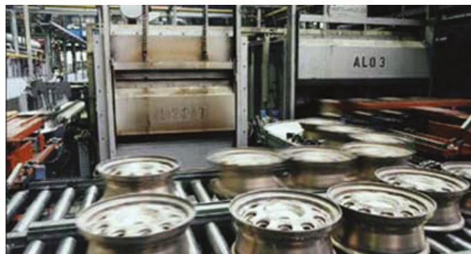
Aluminium age-hardening furnace with air/gas ratio controls for low air pressure protection
