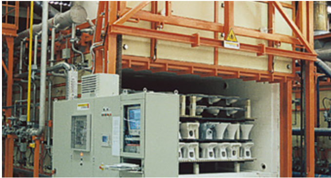
Intermittent shuttle kiln in the ceramics industry
