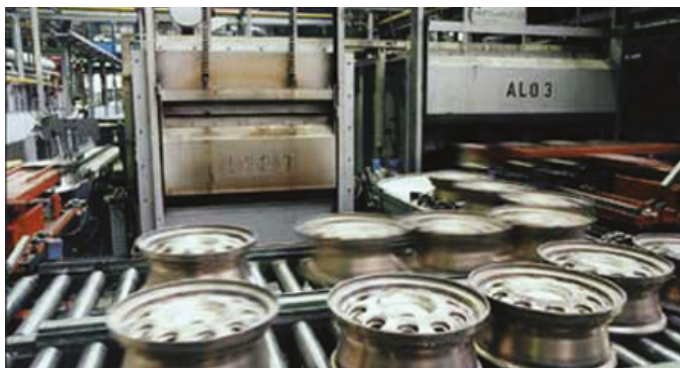
Wheel rim hardening installation
