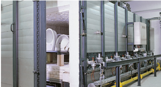
Intermittent shuttle kiln in the ceramics industry
