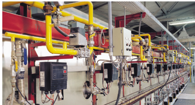
Roller hearth kiln in the ceramics industry
