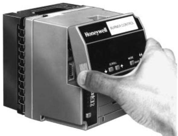
Fig. 9. Keyboard Display Module mounting.
