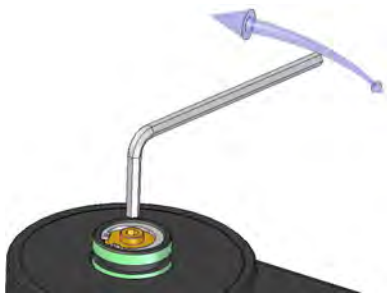
Figure 9 Adjusting flow rate.
