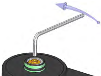
Figure 9 Adjusting flow rate.
