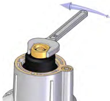
Figure 11 Adjusting flow rate.
