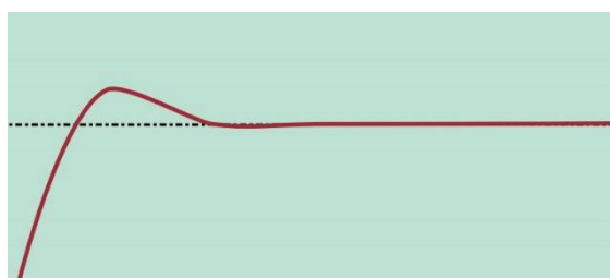
Too Small: Overshoots setpoint before settling
