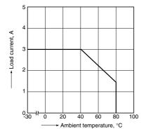
1.-(2) Load current vs. ambient temperature (10 A type) Part No.: AQ10A2-ZT4/32VDC (A) When not using a heat sink
