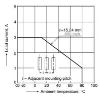
4.-(2) Load current vs. ambient temperature characteristics for adjacent mounting
