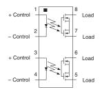
**Switching Characteristics** of Normally-Open (Form-A) Devices
