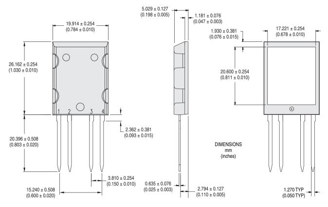
NOTE: Back-side heat sink meets 2500V<sub>ms</sub> isolation to the pins.
