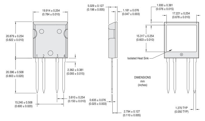
NOTE: Back-side heat sink meets  $2500V_{rms}$  isolation to the pins.
