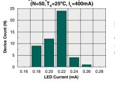
Typical I<sub>F</sub> for Switch Operation
