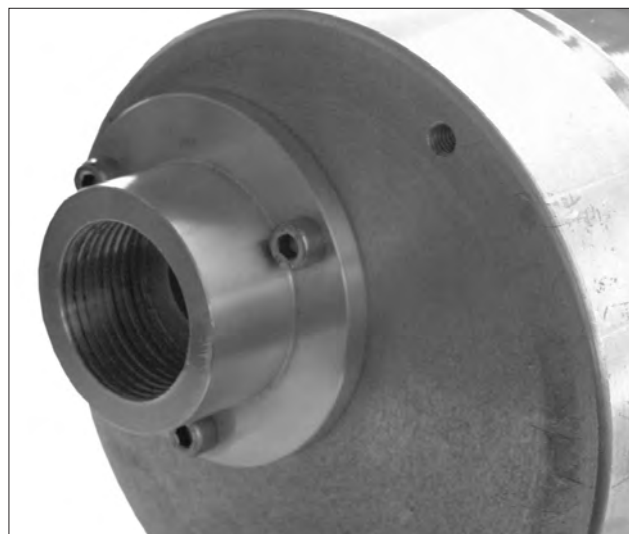
Fig. 9. Mounting the C7061F1xxx detector
